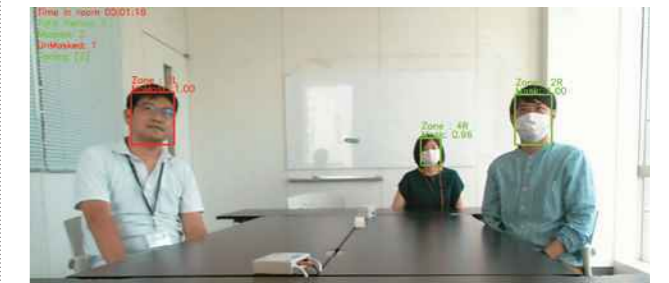
The NRI AI Camera for Office detects that the person at the left side of the screen is not wearing a mask (indicated by the red frame) and gives an audio warning to wear a mask
