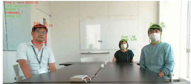
The NRI AI Camera for Office detects that the person at the left side of the screen is not wearing a mask (indicated by the red frame) and gives an audio warning to wear a mask
